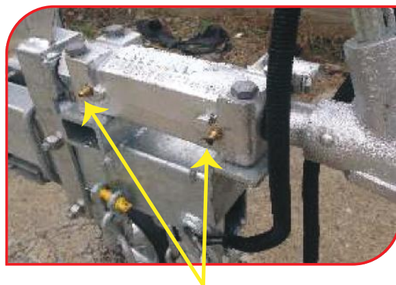
Grease Point on Tow Hitch Grease on regular basis
