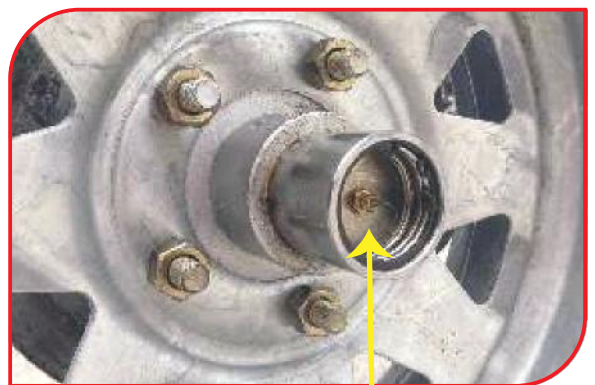
Grease Bearing Buddies, prior to putting trailer in water
